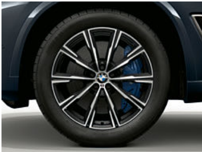
Optional 20" M light alloy wheels Star-spoke style 740 M in Bicolour Orbit Grey with mixed tyres and runflat tyres, burnished, front 9J x 20 with 275/45 R20 tyres, rear 10.5J x 20 with 305/40 R20 tyres.
